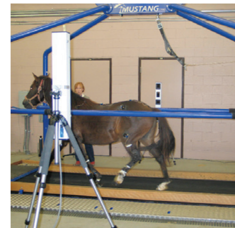
Figure 2. Horse exercising on a treadmill with active motion analysis markers in place to record dynamic fetlock angles.
